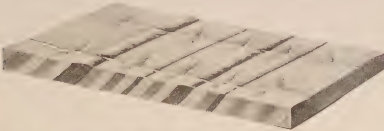
FIG. 91. — One of three diagrams showing the development of topography in a region where the underlying strata are inclined (dip) and vary greatly in their resistance to erosion. The region is conceived to be reduced to a peneplain with low ridges of harder strata. (Modified after Davis.)
